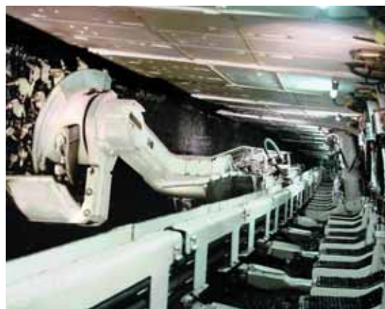
Longwall mining involves the full extraction of coal from a section of the seam using mechanical shearers. Photograph courtesy of Joy Mining Machinery.
